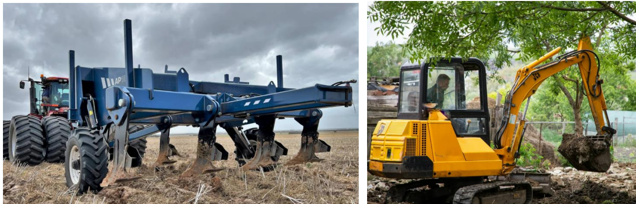
Figure D-9: Shank for deep ripping (left) Toothed bucket backhoe for soil fracturing and de-compaction/(right)
