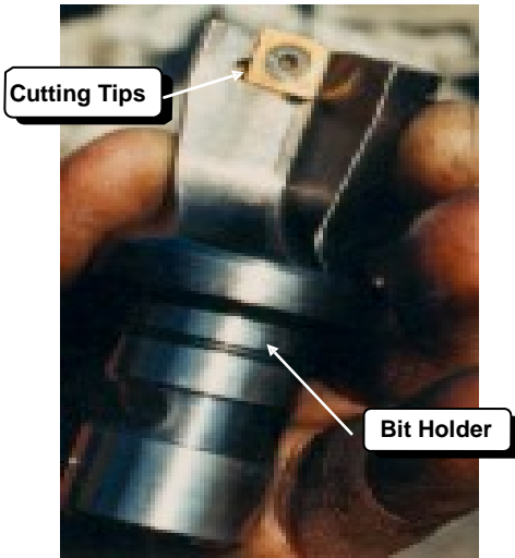
Figure 13. – Carbide Tipped Coring Bit
