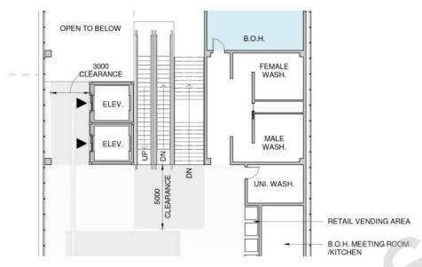
Figure 4-43: Flow-through elevator - Option 2 - Ground floor and transfer level
