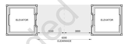
Figure 4-40: Elevator clearance - Plan
