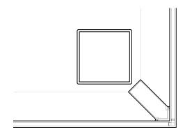
Figure 4-14 - Mullion and Structure alignment at corners
