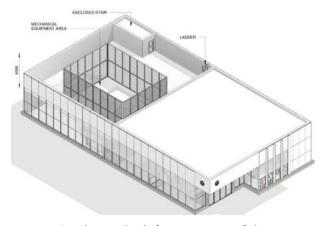
Figure 4-19: Below grade platform station - Roof elements
