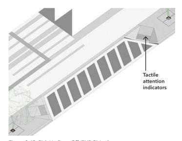
Figure 3-65: Pick Up Drop Off (PUDO) Layby
