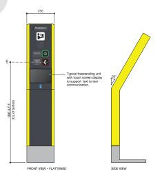
Figure 2-4: DWA Assistance Intercom at platform level Note: Images for visual reference only.
