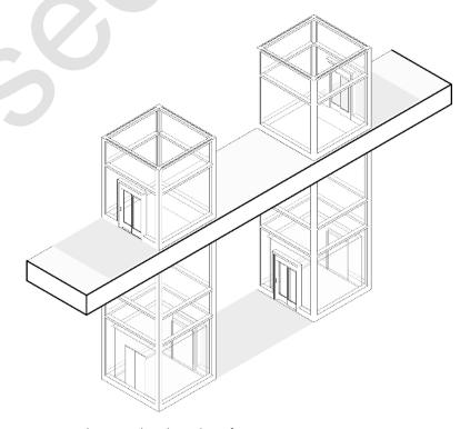
Figure 4-41: Elevator - Flow through configuration - Axonometric
