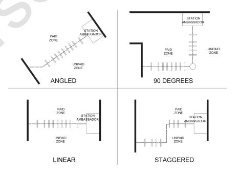
Figure 5-8: Fare gate configurations
