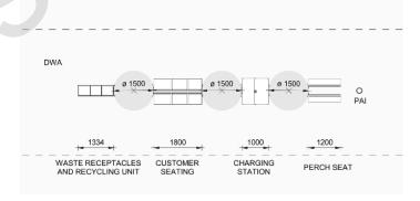
Figure 7-7: Diagram demonstrating the clearances required for DWA and the relationship between the interior elements
