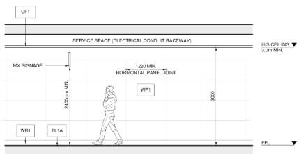
Figure 4-49: Pedestrian tunnel - Longitudinal section
