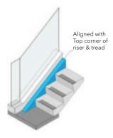
Figure 4-35: Stair - Bike Runnel channel
