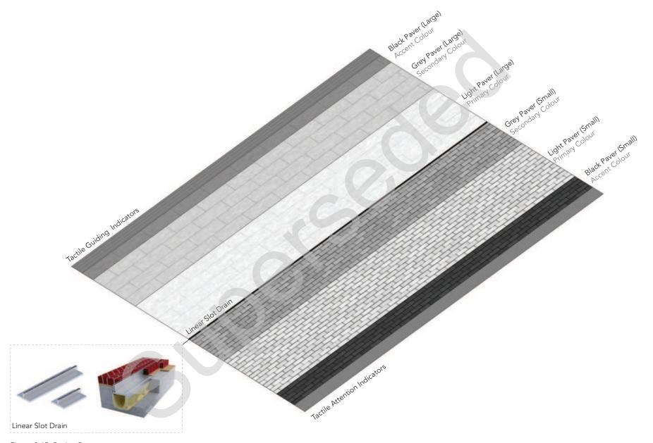
Figure 3-15: Paving Patterns
