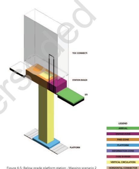
Figure 4-5: Below grade platform station - Massing scenario 2
