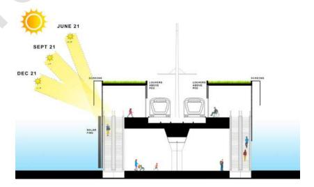
Figure 4-51: Elevated platform station typology - Sun study section
