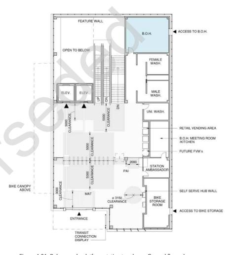
Figure 4-31: Below grade platform station typology - Ground floor plan
