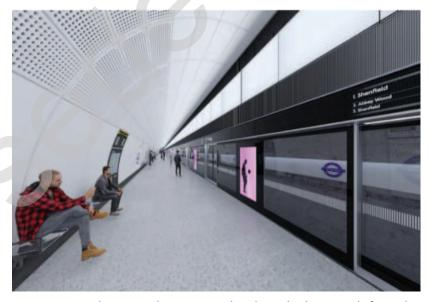
Figure 7-5: Precedent image demonstrating the relationship between platform edge doors, information, digital signage and lighting Elizabeth Line - Transport for London
