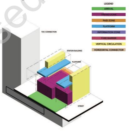
Figure 4-7: Elevated platform station - Massing scenario 4
