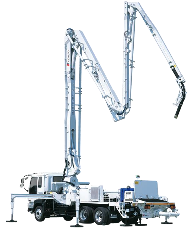
Photo: Example of a Concrete Pumping Truck similar to the one being used on site
