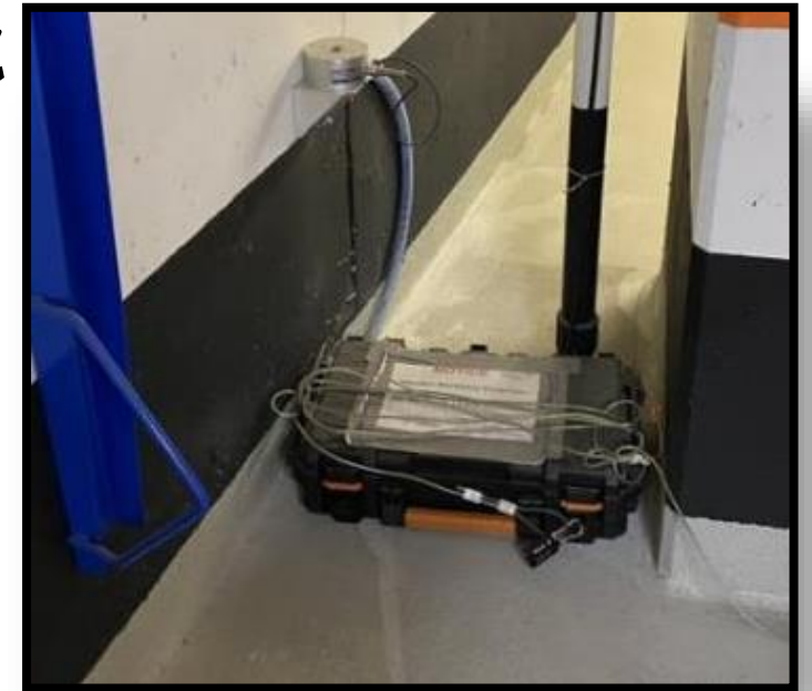
Example of Vibration Monitoring Equipment installed in Union Station
