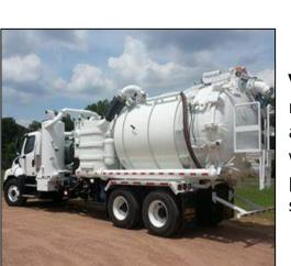
Vacuum Trucks remove dust, debris, and slurry from the work site through powerful suction systems.
