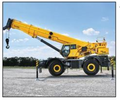
Temporarily stationed on-site during equipment assembly/disassembly, **mobile cranes** lift and move heavy materials, such as steel beam and concrete segments.
