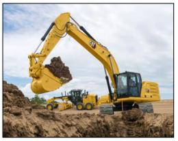
**Excavators** are large, powerful machines used to tear down large sections of structures, including concrete and steel.
