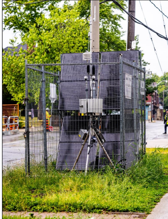
Left to right: A noise and vibration monitor near site, a noise blanket installed on the fencing of the site.
