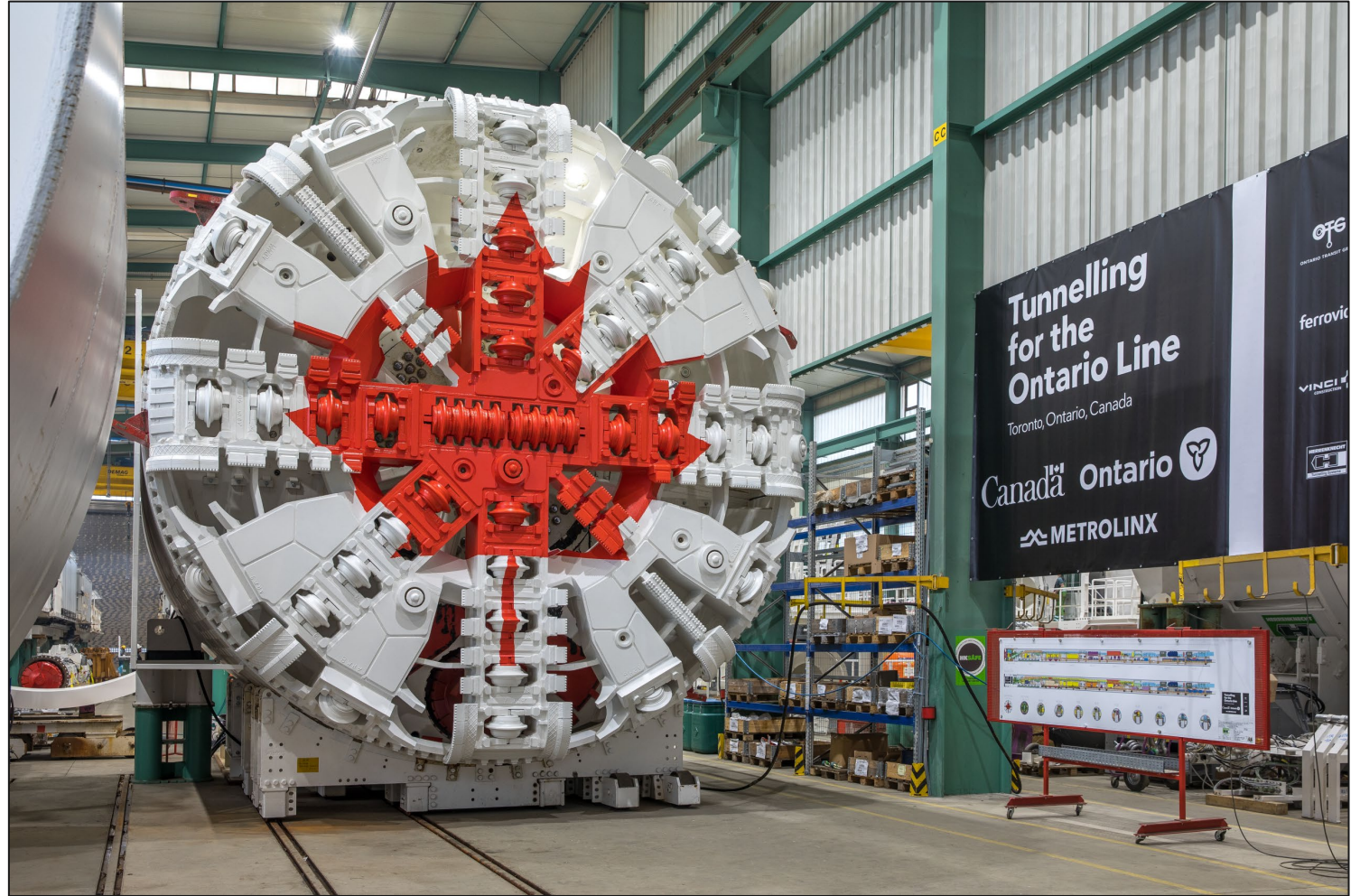
Cutterhead on one of two tunnel boring machines for use on the Ontario Line.
