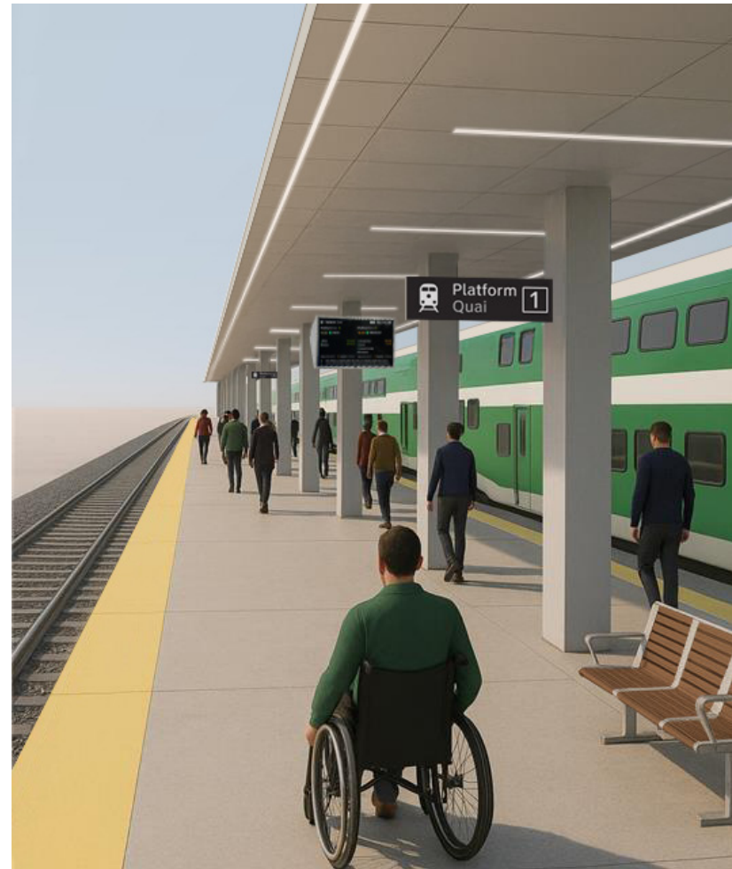
Figure 5-10 Conceptual view of platform area illustrating materiality, and integration of lighting. Lighting design is subject to actual canopy design and photometric analysis.
