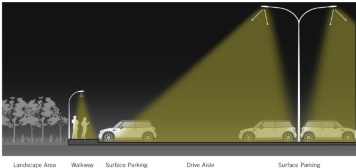
Figure 20: Lighting Design Requirements - Surface Parking
