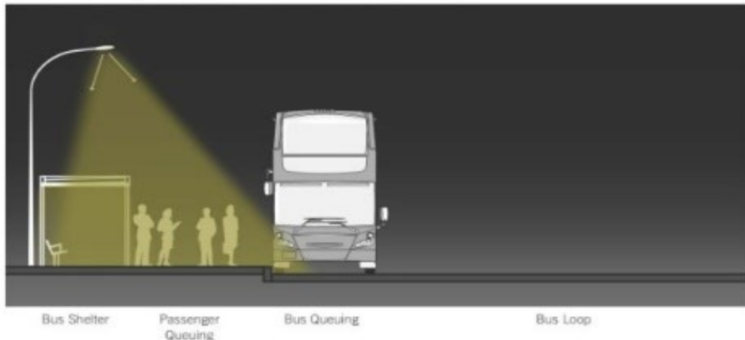
Figure 18: Lighting Design Requirements - Bus Loop
