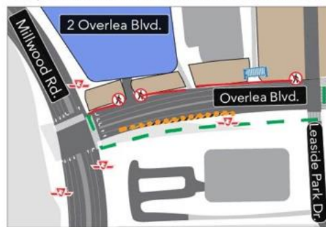
5. Closure of the bike lane adjacent to the eastbound curb lane on Overlea Boulevard east of Millwood Road.
